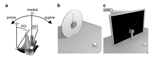
**Fig. 1.** Variables and apparatus. (a) The figure shows the placement of the markers (white squares) and the definition of the forearm and grasp orientation. (b and c) The figures illustrate the setup of Experiments 1 (b) and 2 (c).
