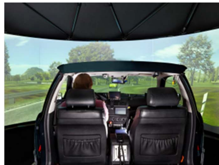
Fig. 1. The WIVW moving based driving simulator. Hexapod movement system (left) and Simulator interior with vehicle mock-up and video projection (right).
